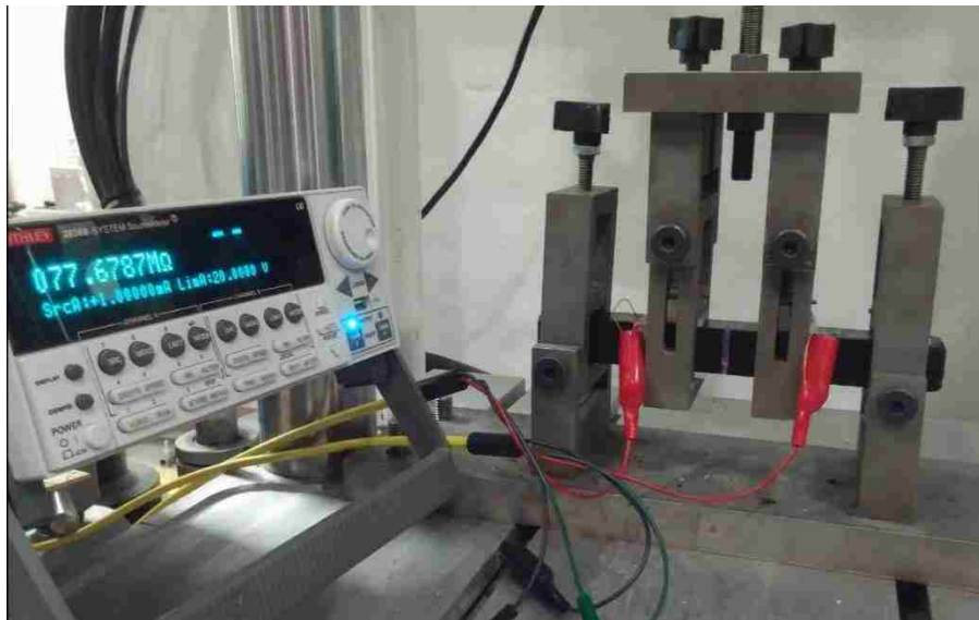
Figure 3.18: In-situ fatigue test showing the loading frame and the source meter connected to measure change in electrical resistance to monitor fatigue damage evolution in PC.
