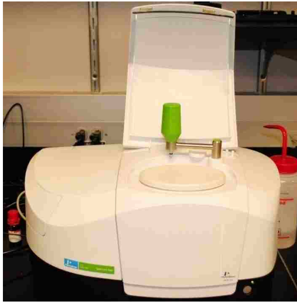
Figure 3.23: PerkinElmer FTIR machine used in microstructural analysis.
